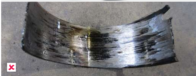
Heavy grooves in the engine mount due to particles in the oil circuit.
