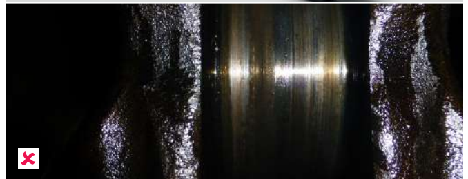
Heavy grooves on the crankshaft due to particles in the oil.
